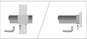
a. Tighten up the grub screws to fix the tube rails in place.
