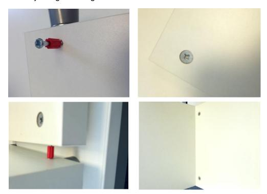
4. Complete the unit with the 'screw caps' and 'hole covers'
