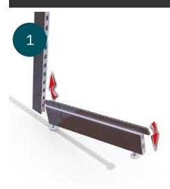
Locate the baseleg rear lug and block into the bottom "H Slots" of the upright as shown.
