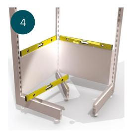
Connect all "L" shaped uprights together by fitting 665mm back panels into the bottom "H slots" of both left and right hand side uprights to the central upright. Now check levels are correct by adjusting the foot discs as required.
