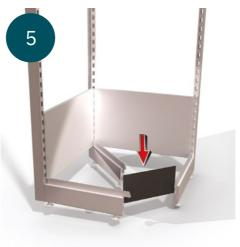
Fit the plinth skirting into position by slotting it between the front capping on the baselegs.
